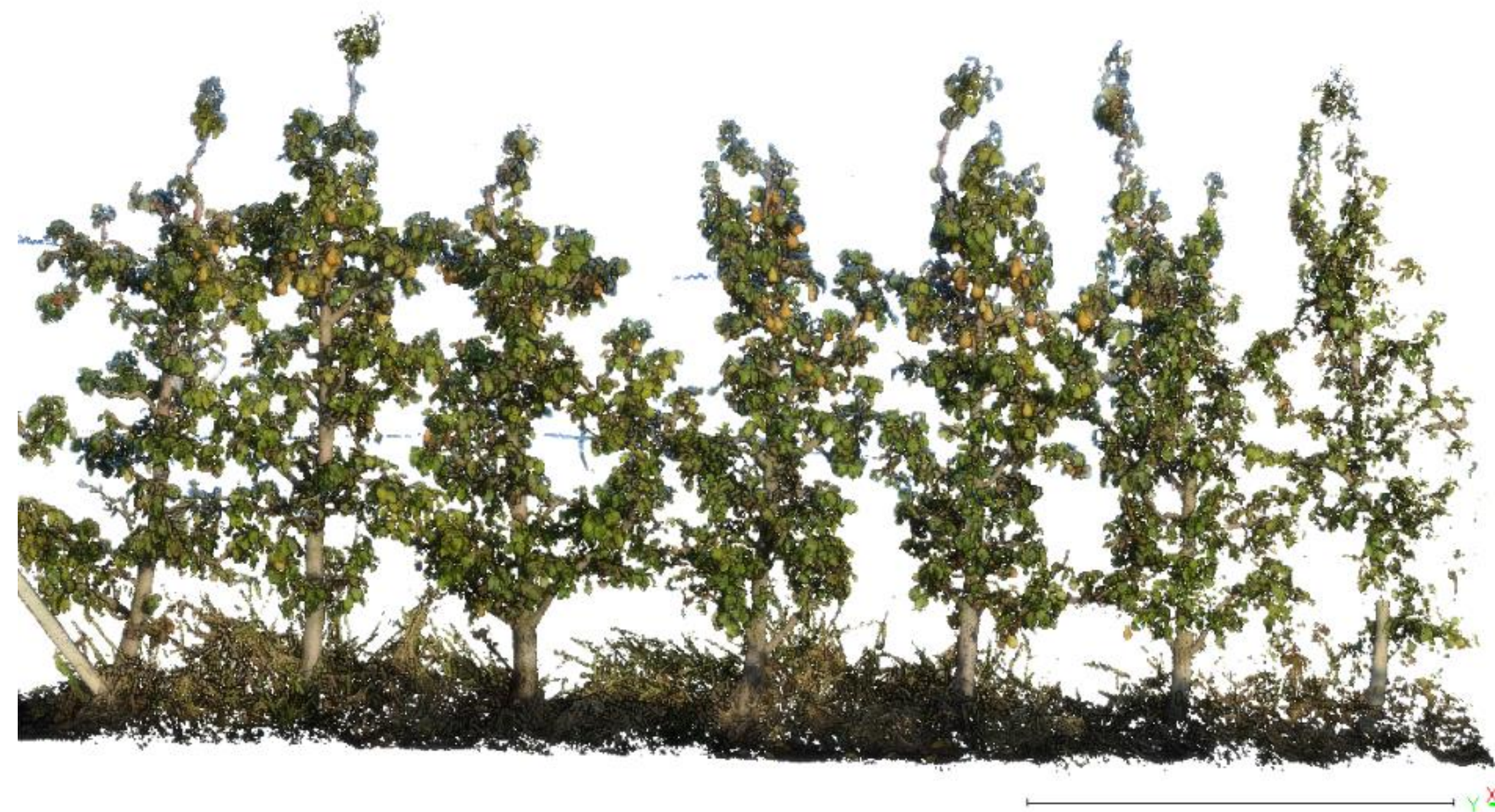
Figure 2. Point cloud created with digital terrestrial photogrammetry with about 82 million points.
