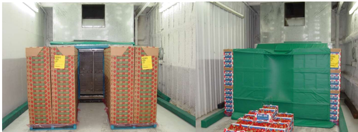
Figure 17. Setup for forced air cooling. Source: Polter's Berry Farm (2019).
