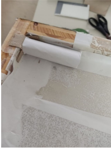
FIGURE 7 | Cylindrical casing for the enclosed air temperature sensor. [Color figure can be viewed at wileyonlinelibrary.com ]
