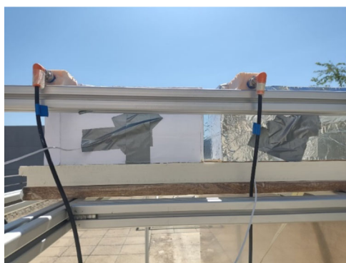
FIGURE 5 | Temperature sensor on the lateral walls of two test boxes. [Color figure can be viewed at wileyonlinelibrary.com ]
