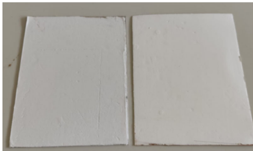
FIGURE 8 | Photography of the sample (copper substrates with CHILLSKYN DRC material). [Color figure can be viewed at wileyonlinelibrary.com ]
