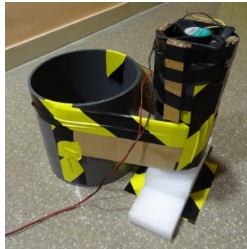
Fig. 3. Acetone evaporator mechanism.
