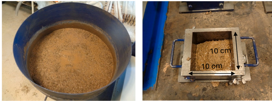
Fig. 2. Appearance of fresh concrete and filling of test specimens.
