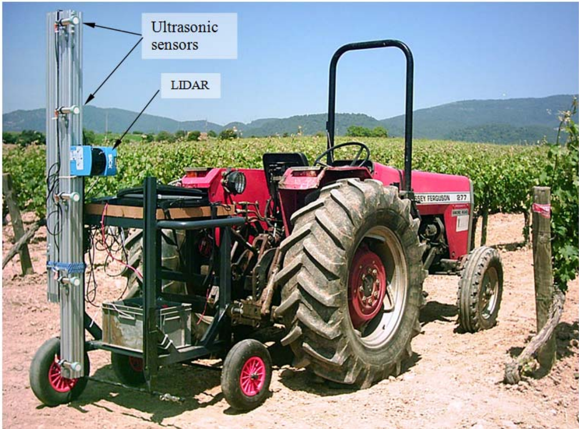
1696 Fig. 4. Ultrasonic and LIDAR sensors mounted on a tractor.
