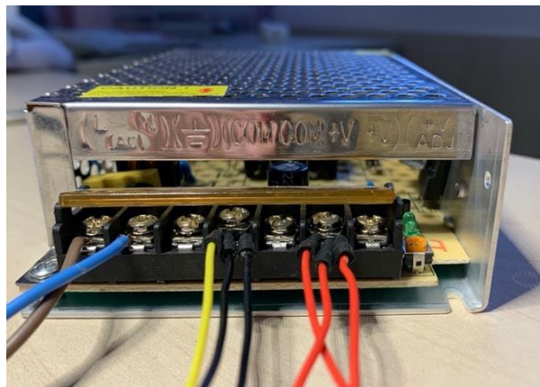
Figure 51: Power supply with three positive and negative cables
