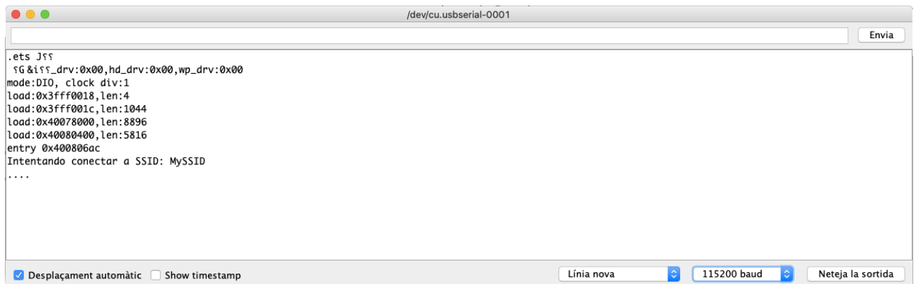
Figure 73: Connection process shown in Ardiono IDE the serial monitor
