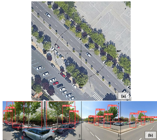
Figure 2: Representation of degrees assignment to ground level and satellite images. a) Tree detection on satellite image and degrees assignment. b) Tree detect in four individual ground level images representing a circumference with degrees assignment.
