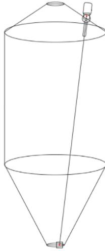
Figure 4: Level Measurement using laser technology
