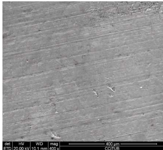
280 Figure 8. SEM superficial study of copper immersed in \text{MgSO}_4 \cdot 7\text{H}_2\text{O} at 130^\circ\text{C} and 20 281 mbar of vacuum pressure during 100 hours 282
