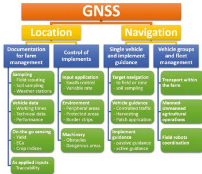
Figure 2: GNSS applications in agriculture (adapted from Auernhammer, H., 2001. Precision farming - the environmental challenge. Computers and Electronics in Agriculture 30, 31-43).
