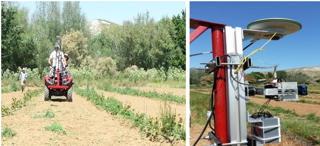
Figure 1. Image of the ATV with a structure to support the terrestrial LiDAR sensor, acquiring data on a field of poplar energy crop (left) and detail of the data acquisition system (right), ready to capture height readings.
