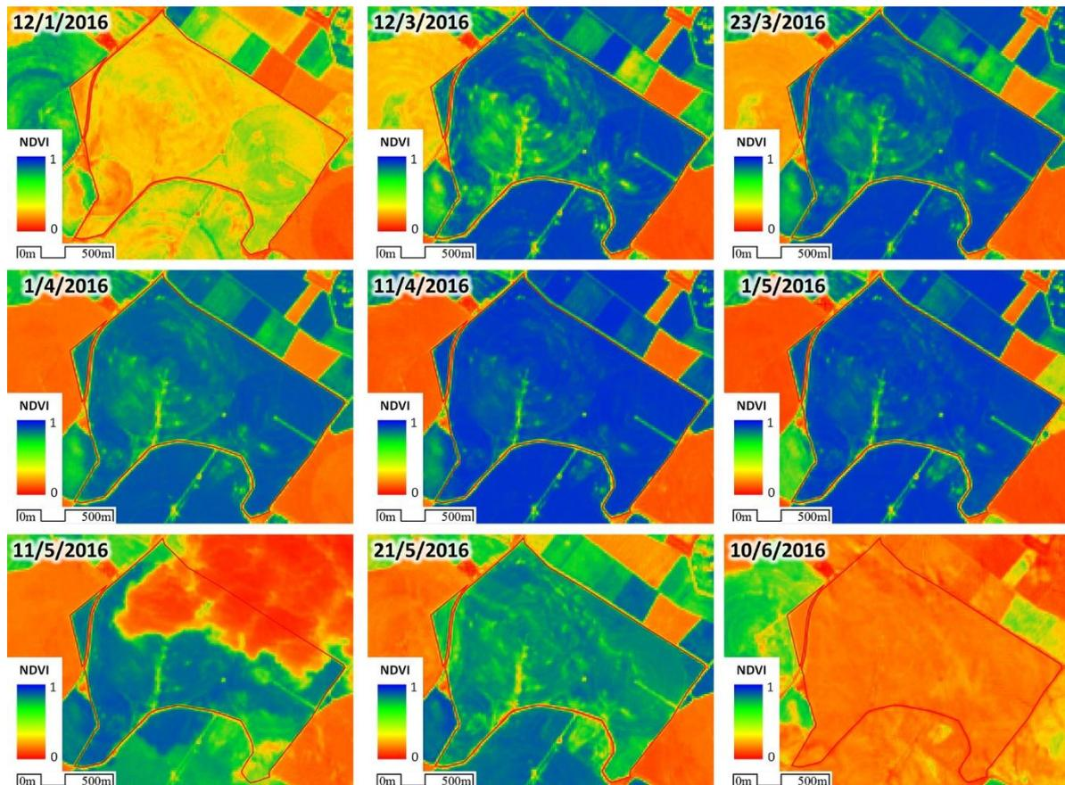
Figure 2. NDVI evolution along the entire season using all available and useful Sentinel-2 products. Images were processed to obtain bottom-of-atmosphere reflectance using the dark object subtraction (DOS1) correction. See digital document for colour information.
