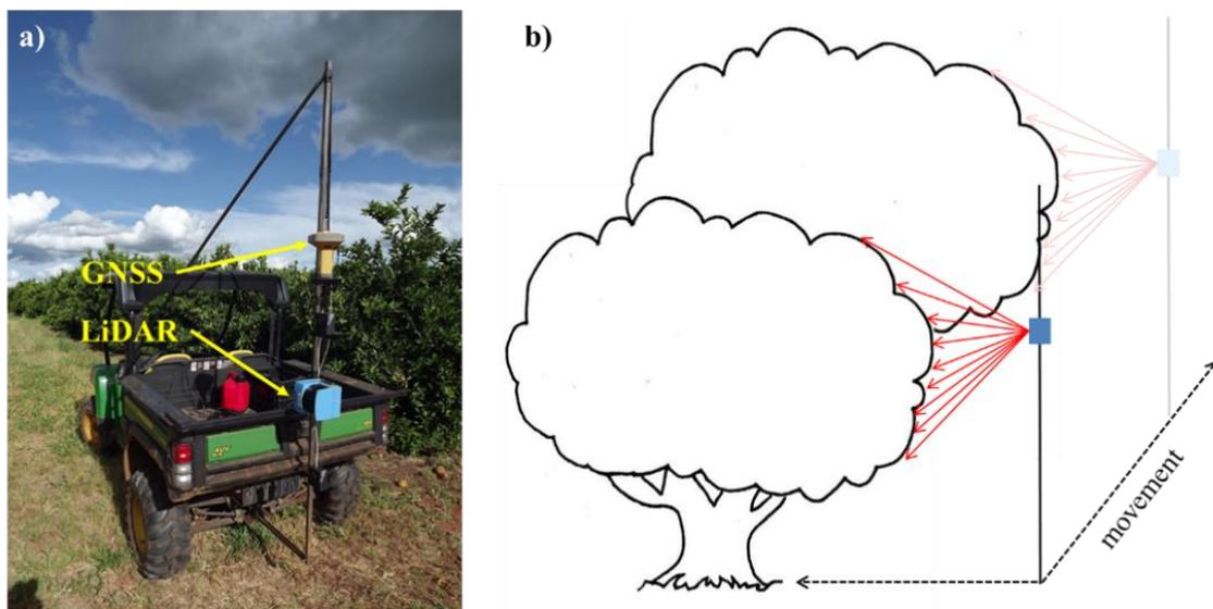
**Figure 1** LiDAR sensor and GNSS receiver mounted on an ATV vehicle (a); LiDAR sensor (in blue) facing the side of the tree row (b)
