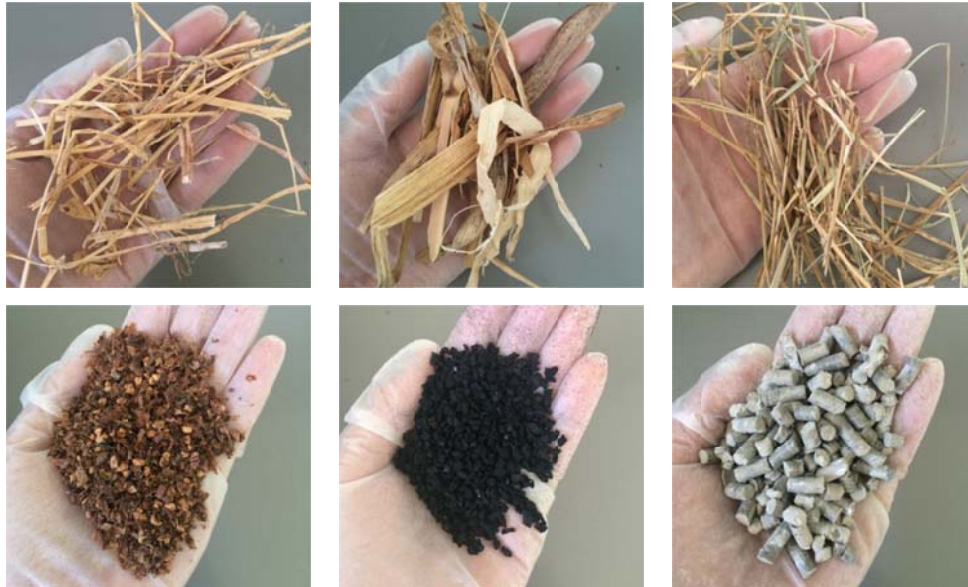
Figure 1. Fibres (up) from left to right: straw, corn plant and fescue. Pellets (down) from left to right: olive stones, rubber crumbs, and polyurethane.
