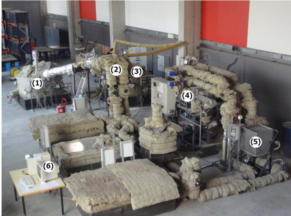
Fig. 2. High temperature pilot plant at University of Lleida, Spain. (1) Hot tank, (2) HTF-salts heat exchanger, (3) Cold tank, (4) Electrical boiler, (5) HTF-air heat exchanger, and (6) acquisition and recording system
