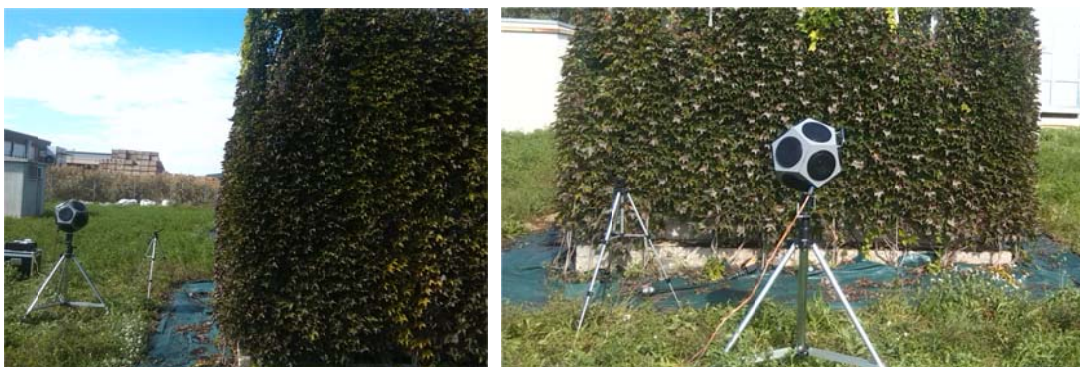
Figure 7. In situ acoustic measurements according to UNE-EN ISO 140-5
