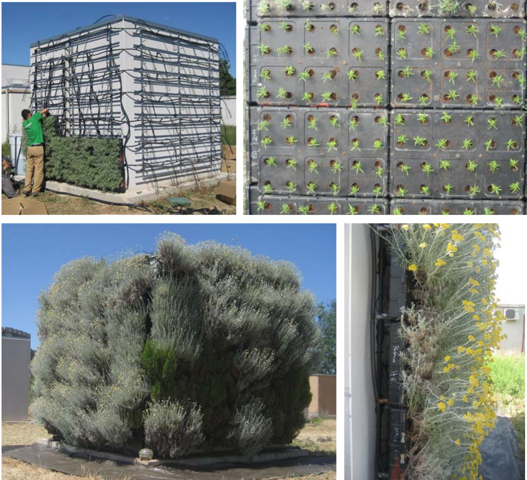
Figure 5. Green Wall made with polyethylene modules, coconut fibre substrate and native shrubs
