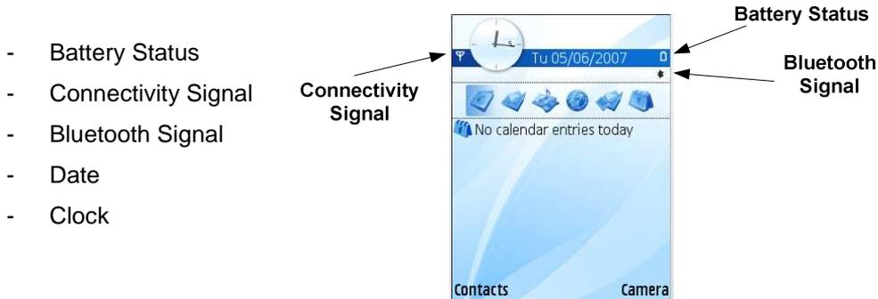
Figure 20: Main screen of the Operating System Symbian S60
