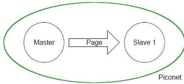
Figure 10: Point-to-Point Connection
