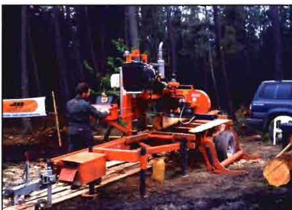
F.13. Miniserradero transportable Wood-Mizer.
