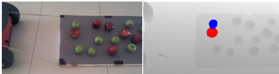
Figure 9: Example where K-Means is used to separate two close fruits. Highlighted in red and blue two fruits too close from each other.
