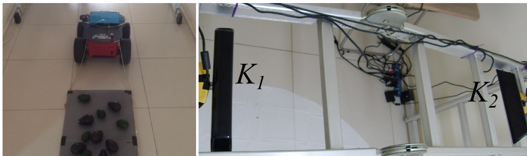
Figure 14: Experimental Setup. Left image shows the mobile robot carrying fruits and right image the kinects mounted in a metal structure. The Kinect in the left corresponds to the sensor K_1 and the Kinect in the right correspond to the sensor K_2 .
