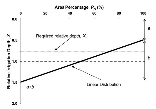
Fig. 1. A linear water application model for micro-irrigation; X, relative irrigation depth;  $P_A$ ,
