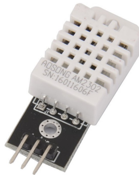
Figura 1: Sensor de temperatura i humitat, model DHT22
