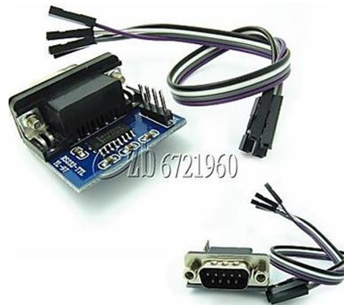
Figura 8: Conector RS-232 Externo
