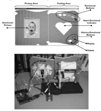
Figure 3: Picture frame enhanced with emotion sensors and expression systems (front and rear views)
